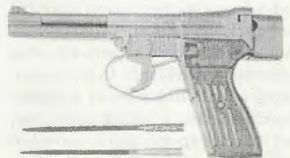
Ammunition technology similar to Underwater Assault Rifle makes 4.5mm Underwater Pistol effective close-quarters weapon, with lethal range of 17 meters underwater, or 50 meters above water. Featuring four barrels and double-action firing mechanism, SPP-1 is simple to load, operate.
